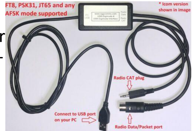
Built-in USB Sound Card and USB CAT control Isolated audio and PTT - CAT uses FTDI UART
